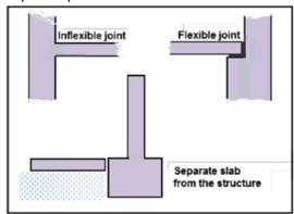
Examples of flexible versus inflexible structural design used to prevent building damage caused by expandable clay
