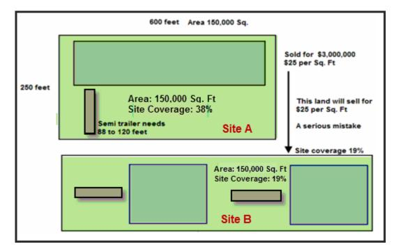
The impact of the turning radius of semi-trailers on the building layout, site coverage and land value.
